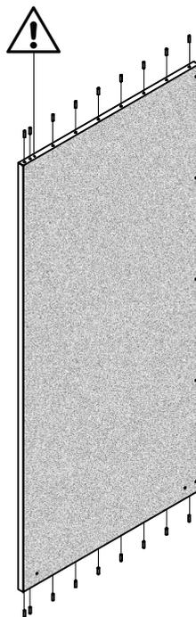
[EN] **Vacuum or blow out the holes for the wooden dowels in the side walls, ceiling and floor. Then you need to insert 9 wooden dowels (002) into the pre-drilled holes on the upper and the lower side of right side wall and the left side wall. For the back wall, please insert 6 wooden dowels (002) on each side. When resting the walls on the dowels, please be careful not to break the dowels. Ideally put some cardboard underneath.**
